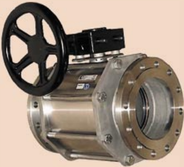
Full-hole DN200, ball and metallic gaskets with hard chrome plating. For high temperatures and abrasive medium.
